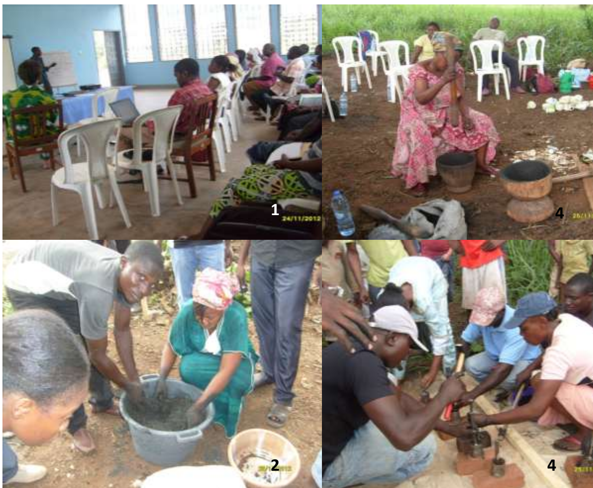
Photo 1: Theoretical training Day 1; Photo 2: Application phase (day 2 and 3) Crushing wood charcoal bits and carbonized agriculture refuse; Photo 3: Mixing sawdust and charcoal powder with binder before pressing into briquettes; Photo 4: Using molds to press mixture into briquettes
