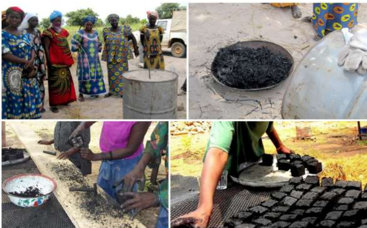
(From top left to bottom right) 1. Pyrolysis training; 2. Carbonized rice-straw; 3. Briquette pressing; 4. Briquette drying
