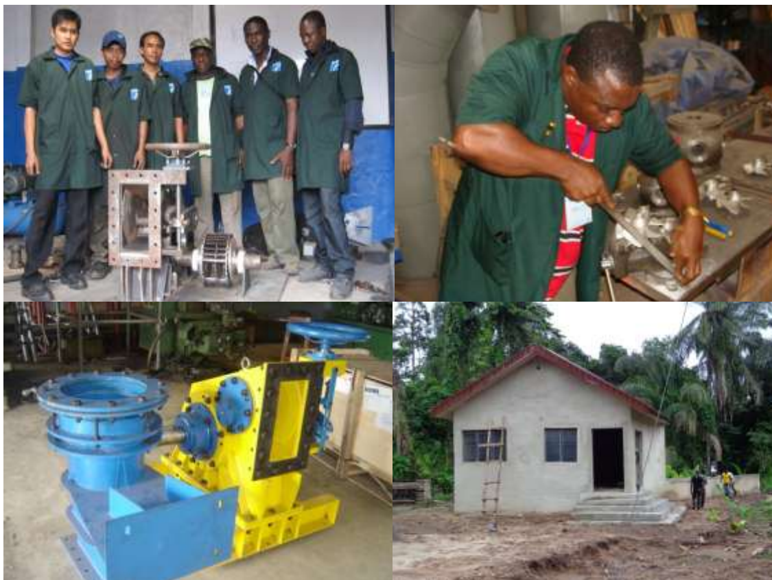
Indonesia: Turbine housing and runner; Indonesia: Turbine manufacture; Fabricated CrossFlow turbine in EMDI
